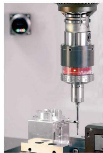
▲ Wireless workpiece measurement, no cover issue
